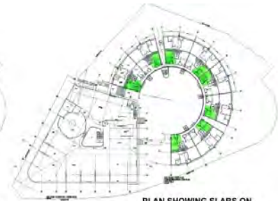
PLAN SHOWING SLABS ON INTERMEDIATE UNIT FLOORS BEING DEMOLISHED TO CREATE DOUBLE VOLUMES
