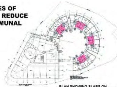
PLAN SHOWING SLABS ON ENTRANCE FLOORS CONVERTED TO COVERED TERRACES
