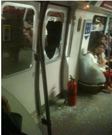
Picture 1: Glass broken by Fire Extinguisher
